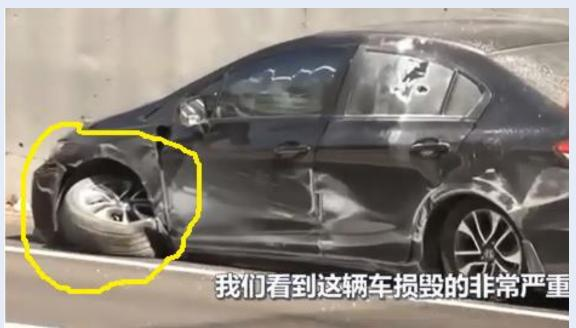
In other words, the car only had three wheels on the ground and is therefore out of control.
